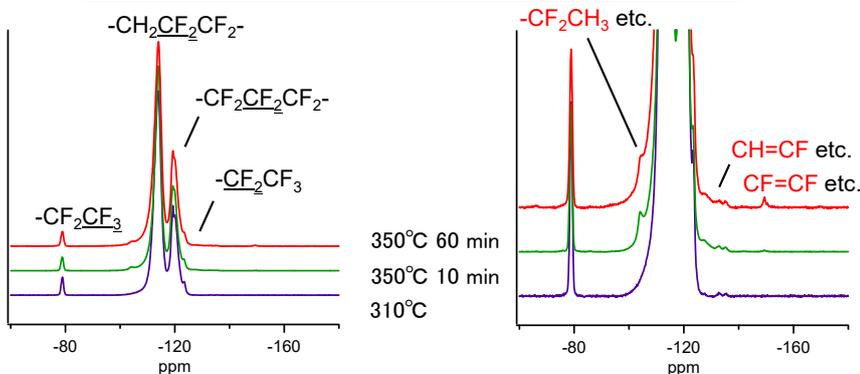
It is considered that C=C and -CF<sub>2</sub>CH<sub>3</sub> are formed. Further detailed information such as the copolymerization ratio can be obtained by <sup>13</sup>C NMR.
