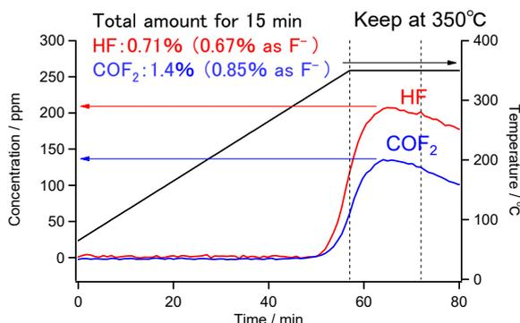
HF and COF<sub>2</sub> were detected separately, and the total amount of the decomposed gas can be estimated. This on-line analysis reveals that the decomposition of this sample begins at 320°C.
