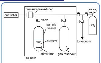
The CO<sub>2</sub> adsorption amount of the sample is determined by introducing CO<sub>2</sub> into the apparatus at a predetermined pressure, then subtracting the CO<sub>2</sub> amount in the empty part of the sample vessel from the incremental weight.
