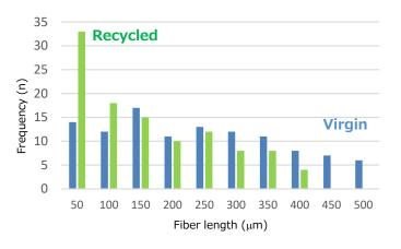
✓ Recycled material A has a higher proportion of short fibers than virgin material
