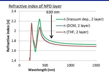
Comparison of refractive index and extinction coefficient
