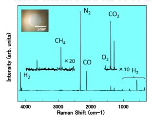
N<sub>2</sub> is process gas in LCD manufacturing, and CH<sub>4</sub>, CO, CO<sub>2</sub>, H<sub>2</sub> are decomposition of organic compounds in LCD panel
