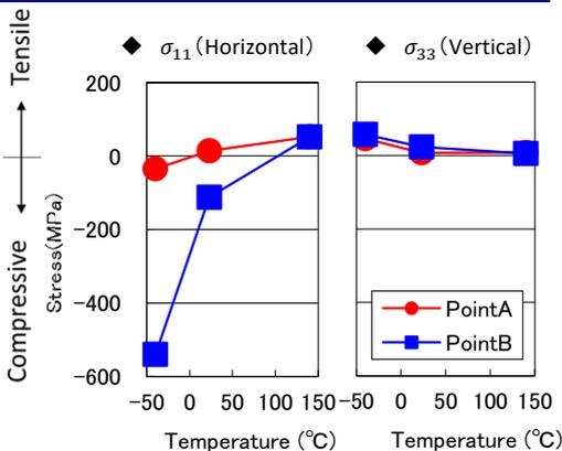
The horizontal stress was largely changed by the temperature. This tendency was remarkably observed at Point B which is located near the solder.
