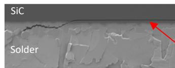
SEM image near the interface between the SiC and the solder after 30 cycles.
