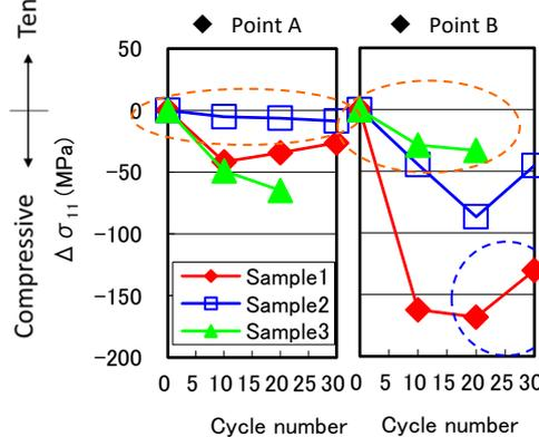
Temperature-controlled heating and cooling stage was used. Cycle range: -40 °C  $\leftrightarrow$  140 °C
