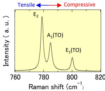
An example of Raman spectra of 4H-SiC ( $\sigma$ -plane).
