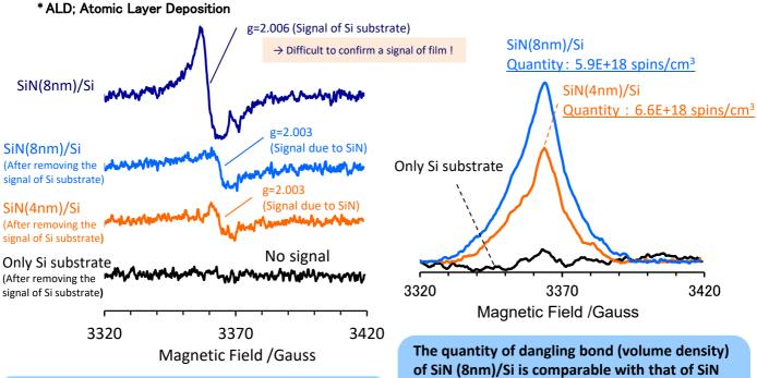
After the signal removal treatment, there is no signal on "Only Si substrate", but the signals of SiN can be clearly confirmed on the ultrathin films. of SiN (8nm)/Si is comparable with that of SiN (4nm)/Si (within ± 10% of quantitative error).
