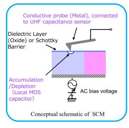
The capacitance of the depletion beneath the probe can be detected as a dC/dV signal. The signal depends on carrier type and concentration.
