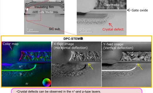
⇒Structure, crystal defect and p-n junction can be characterized
