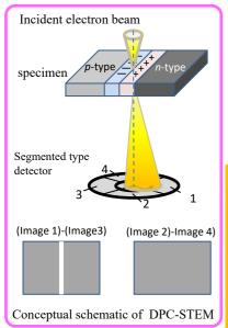
The internal electric field of the p-n junction deflects the incident electron beam. Using the segmented type detector, the variation of the beam deflection appears as a variation of contrast in the image
