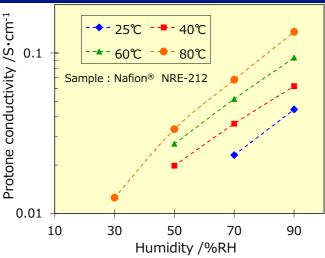
Proton conductivity increases as temperature and humidity increase.
