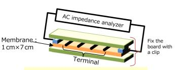
Method: 4-terminal method Direction: Planar direction Frequency: 10 kHz
