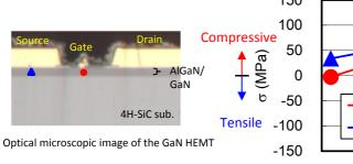
The compressive stress became large at both measurement points as the temperature increased
