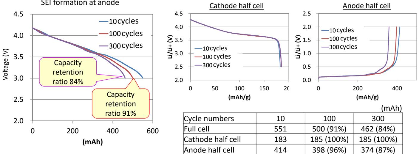
(): capacity retention ratio against 10 cycles
