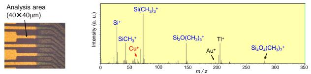
Although the wiring surface is plated with Au, Cu was detected. It means that Cu has migrated from under layer.
