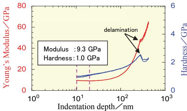
Modulus of a ultrathin film can be estimated by approximate equation. Folding point (arrow in the figure) indicates the comparative evaluation of the adhesion between film and substrate<sup>1).</sup>
