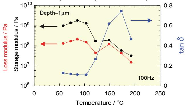
Viscoelasticity at high temperature can be obtained using NI. This method is beneficial for characterization or degradation analysis of thin film, micro material, and specific micro area.
