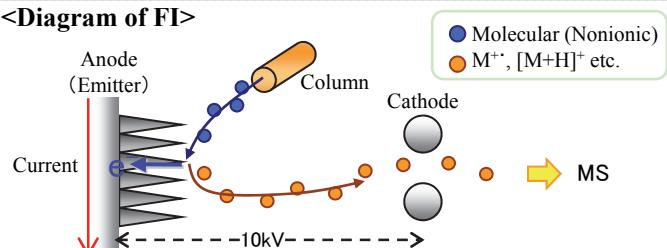
The analyte molecules are ionized by electron tunneling at the tip of the emitter.
