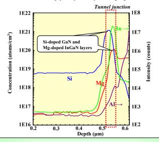
Simultaneous detection of Mg and Si • High sensitivity for Mg
