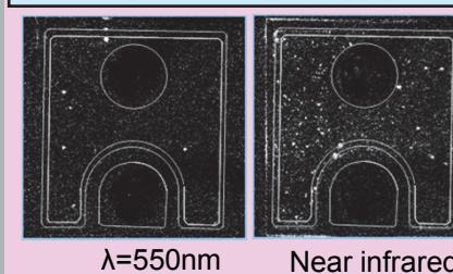
Spectroscopic EL Images of blue LED chip under low current condition.
