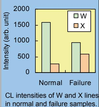
CL measurements were done on the cross-section of IGBTs. Point defects were remarkably changed. The tetra-interstitials (X) were increased and the tri-interstitials (W) were decreased in the failure sample. We consider that the minority carrier lifetime in the failure sample is elongated by the decrease of total number of defects by the agglomeration of interstitials.
