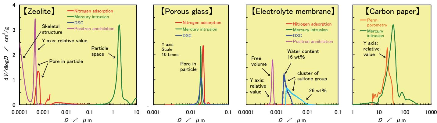
Micro-pores in zeolite or activated carbon → Nitrogen gas adsorption
