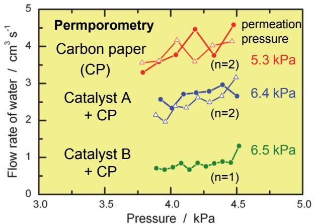
Carbon paper shows the highest permeability and the lowest permeation pressure. On the other hand, water permeability of the catalyst A is higher than B, although water permeation pressure of two catalyst layers (A,B) is almost same. Further investigation including contact angle etc., is needed to reveal the reason for the difference between them.
