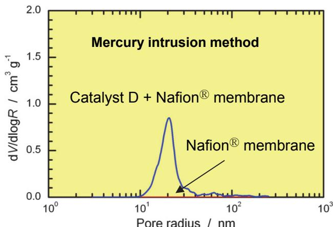
The pores (clusters) in the electrolyte membrane are not detected by mercury intrusion method, we can determine the pore size of catalyst as painted on membrane. If the thickness of the catalyst layer can be measured by SEM, it is also possible to calculate the porosity of the catalyst layer.
