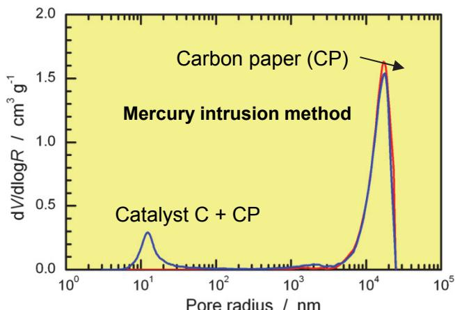
The pore size distribution curve of the catalyst layer (the particle space of carbon) and that of CP doesn't overlap, we can determine the pore size of the catalyst. However, since the pore size of the microporous layer and the catalyst layer overlap, it is necessary to be careful in interpreting the results.
