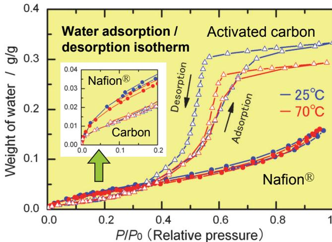
Nafion® has a large amount of water vapor adsorption at low relative pressure (see enlarged view). It is considered that a large amount of water is adsorbed to the hydrophilic sulfone group. The amount of adsorption of activated carbon rapidly increases at high relative pressure, which is presumed to be due to the infiltration of water into nanopores.
