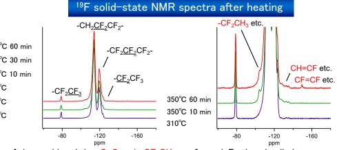
It is considered that C=C and -CF<sub>2</sub>CH<sub>3</sub> are formed. Further detailed information such as the copolymerization ratio can be obtained by <sup>13</sup>C NMR.
