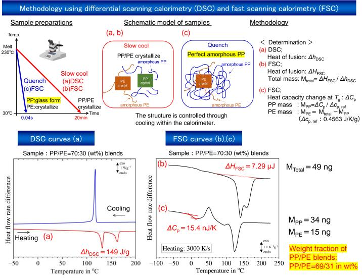
The compounding mixing ratio of PP/PE and the thermal analysis method are consistent (a standard deviation of present method was 1 wt%)
