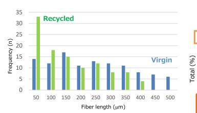
✓ Recycled material A has a higher proportion of short fibers than virgin material
