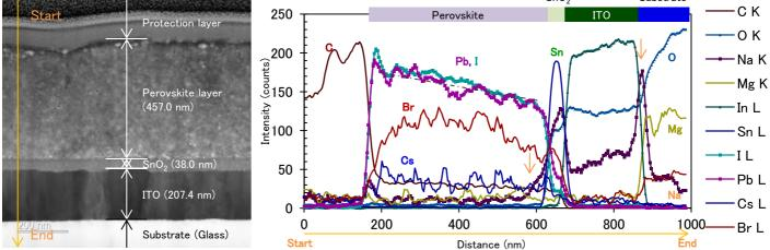
It was detected that the intensity of Pb and I elements on the surface-side of the perovskite layer was higher than that of the inside, and the intensity of Na element was high at ITO/ substrate interface. Heating behavior of materials can be observed from room temperature to 1300°C by in-situ TEM observation.
