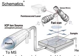
Inorganic elements in aerosol which generated by irradiating laser on a solid sample are analyzed by ICP-MS.
