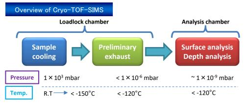
Surface analysis & depth analysis of samples which include much volatile components are possible by cooling samples to appropriate temperature.
