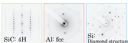
Fig.5 : Selected area electron diffraction patterns
