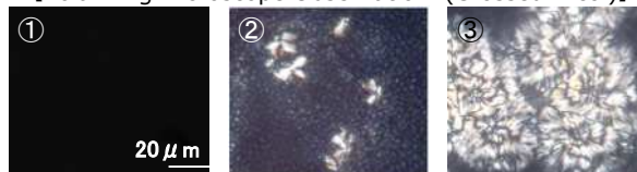
① amorphous, ② & ③ Spherulites in different size observed
