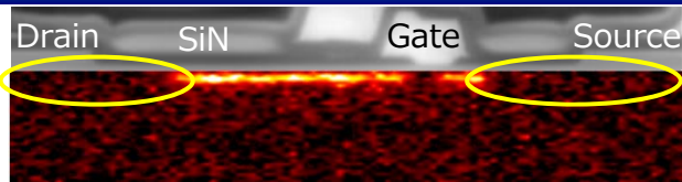
CL image of AlGaIn (20 nm) layer at \lambda=320 nm.
