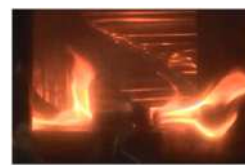
Over charging test of cylindrical battery
