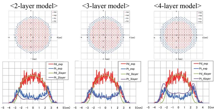
The number of shell layers is determined in an atomic level by fitting core-shell models and experimental EDX profiles. \*
