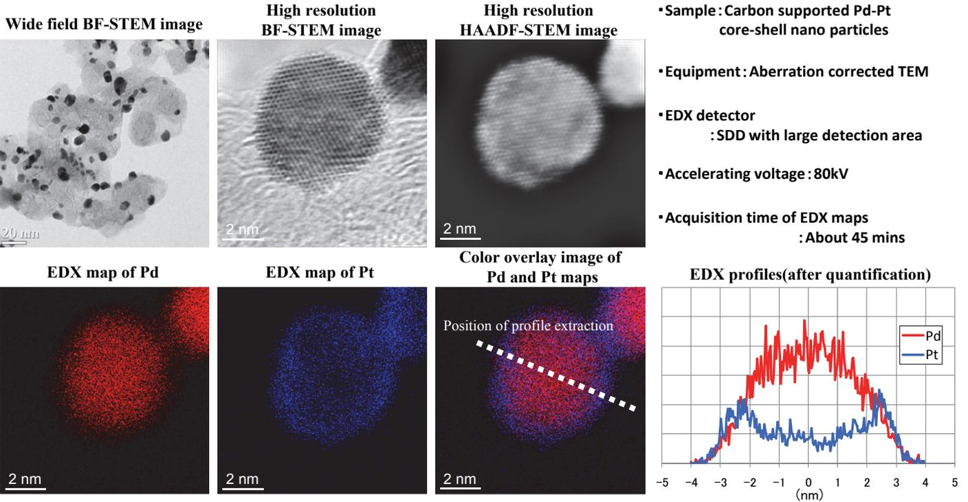
Clear elemental maps of small nanoparticles about 5nm in size can be acquired by combination of aberration correction, high sensitive EDX analysis, and low accelerating voltage measurement (80kV).
