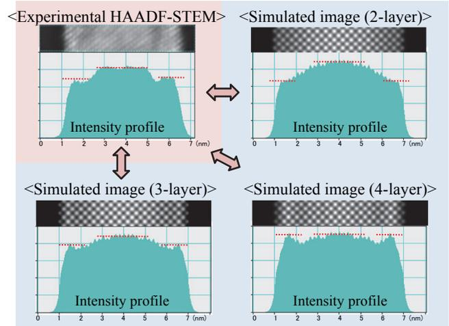
Results of the HAADF-STEM image simulations show the 3-layer model is similar to the experimental data.
